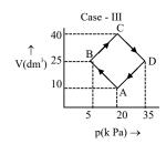
An ideal gas undergoes a cyclic transformation starting from the point A and coming back to the same point by tracing the path  $A \rightarrow B \rightarrow C \rightarrow D \rightarrow A$  as shown in the three cases above.
